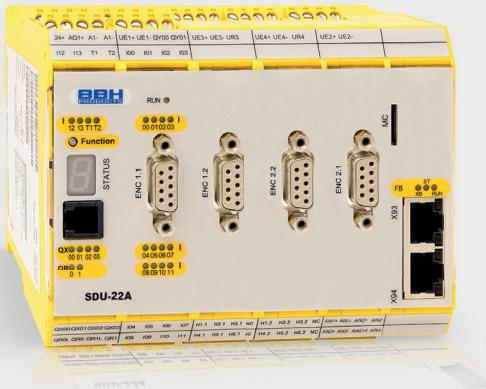
FSoE slave module for safe speed and position of up to 2 axes for further evaluation in an FSoE master module
