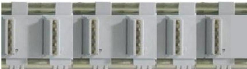
There is no TB2 between the last SMX121-2 module and the communication module SMX5x because the power supply for the SMX5x is fed in through the backplane bus system.
