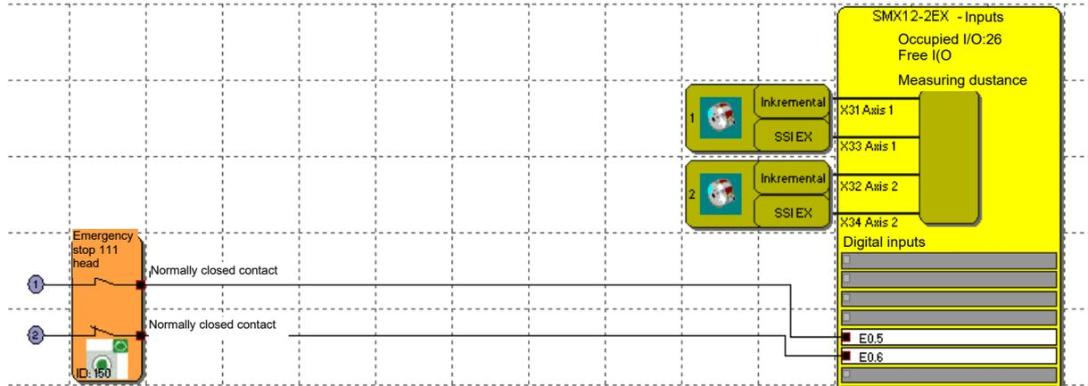
Emergency stop contacts from emergency stop relay with pulsing from the **SMX100**
